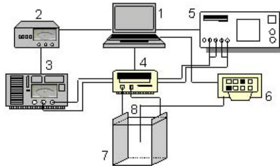
Figure 1 Schematic diagram of Ohmic heating and electrical impedance measurement system: 1) PC, 2) signal generator, 3) bipolar amplifier, 4) switch unit, 5) impedance analyzer, 6) data logger, 7) coagulation vessel, 8) thermocouple
