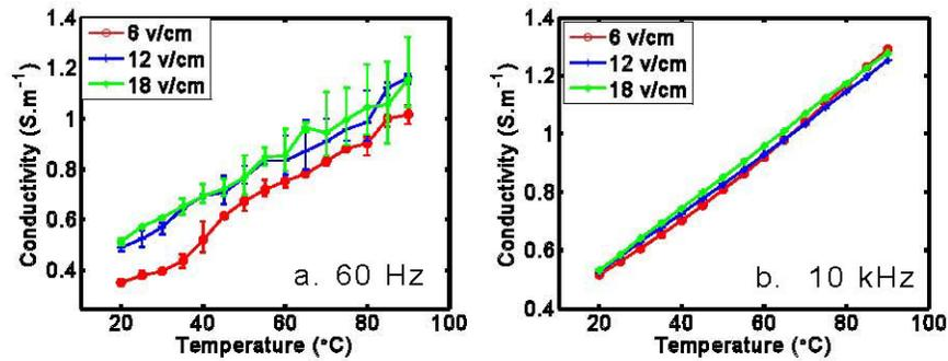
Figure. 4 Electrical conductivity of soymilk-coagulant mixture at three electric field strength 6, 12, 18 V/cm at frequency a. 60 Hz and b. 10 kHz.
