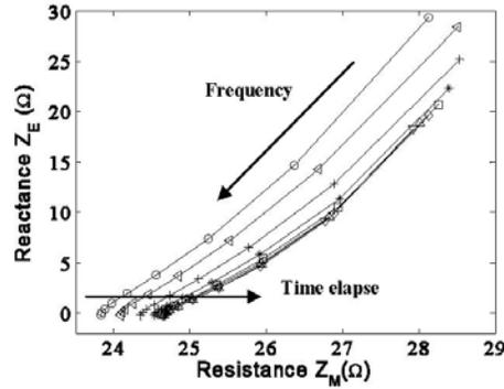
Figure 6 Cole-Cole plot at various coagulation time. Coagulation time 0 min (O), 3 min ( $\diamond$ ), 10 min (+), 20 min (\*), 30 min ( $\square$ ), 40 min ( $\diamond$ ), 50 min ( $\triangle$ ), 60 min ( $\nabla$ ).
