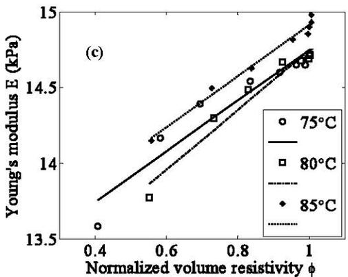
Figure 11 Correlation between volume resistivity and rheological properties at various temperature, (a) apparent breaking stress, (b) apparent breaking strain and (c) apparent Young's modulus
