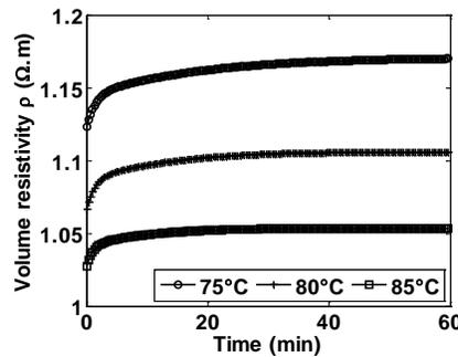
Figure 7 Time variation of volume resistivity (at 10 kHz) at 75, 80, 85 C during coagulation.
