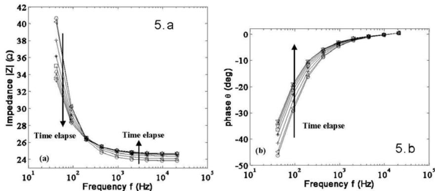
Figure 5 Bode diagram of variation of impedance (5.a) and phase (5.b) with the progress of coagulation at 80 C.: coagulant time 0 min (O), 3 min (◁), 10 min (+), 20 min (\*), 30 min (◻), 40 min (◊), 50 min (△), 60 min (▽).
