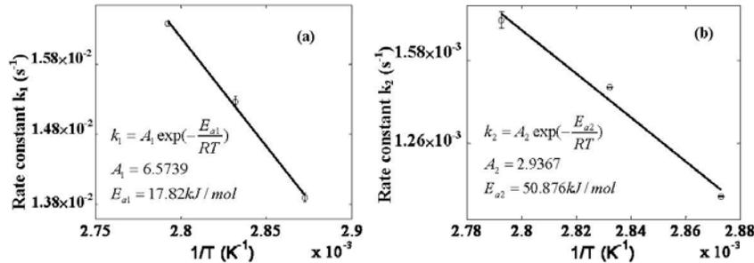
Figure 9 Arrhenius plot of the rate constants for the two stages of coagulation process: (a) rate constant  $k_1$  of the first stage,  $r=0.998$  (b) rate constant  $k_2$  of the second stage,  $r=0.992$
