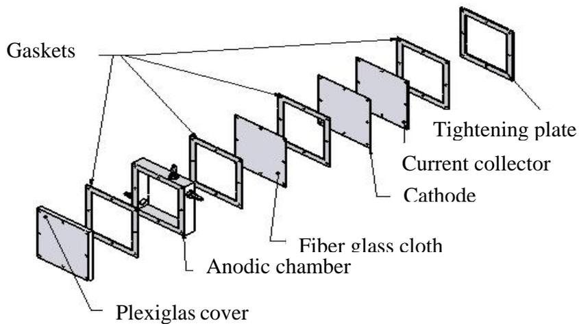
**Figure 1. Single chamber MFC exploded view.**
