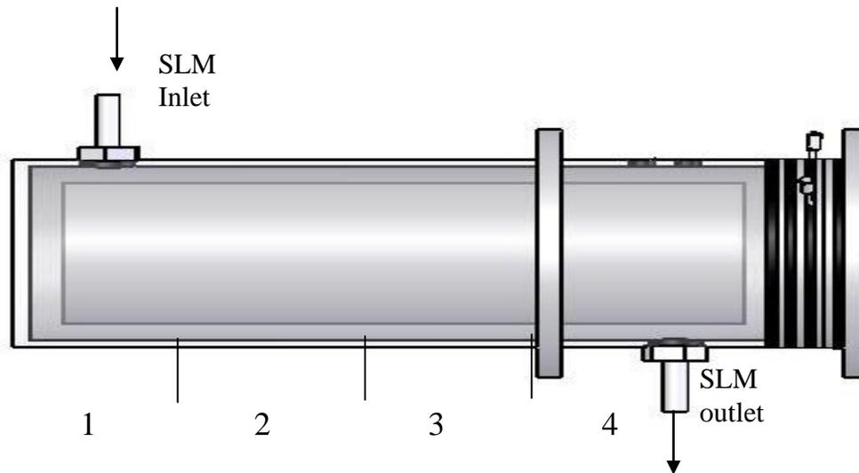
**Figure 3. Dual chamber MFC sampling zones**
