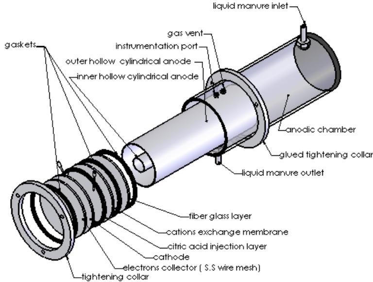
**Figure 2. Dual chamber MFC exploded view.**
