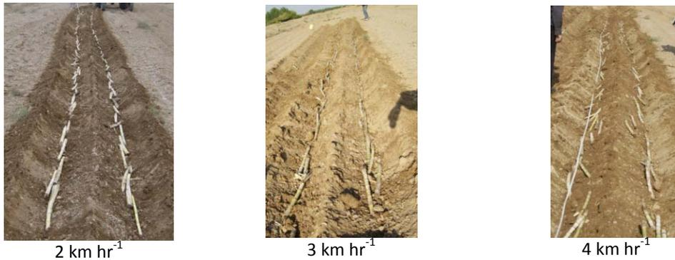
Figure 4. Effect of forward speed on uniformity of planting
