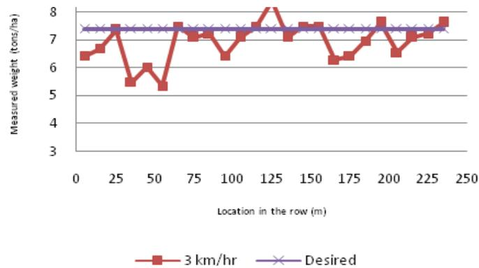
Figure 9. Uniformity of planting at 3 km hr<sup>-1</sup> forward speed compared with desired level of billet consumption
