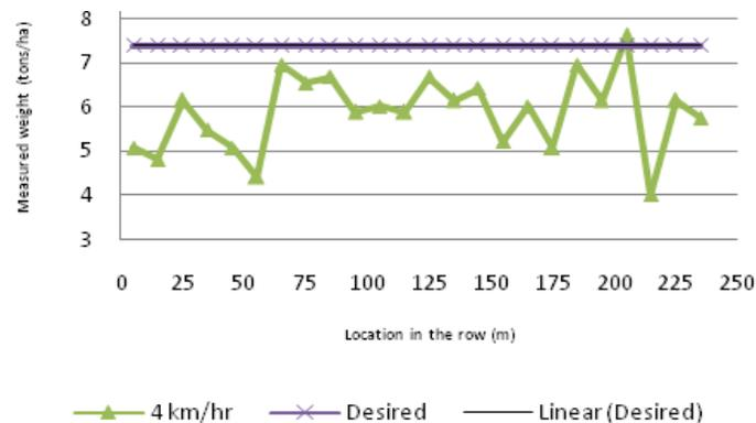
Figure 10. Uniformity of planting at 4 km hr<sup>-1</sup> forward speed compared with desired level of billet consumption
