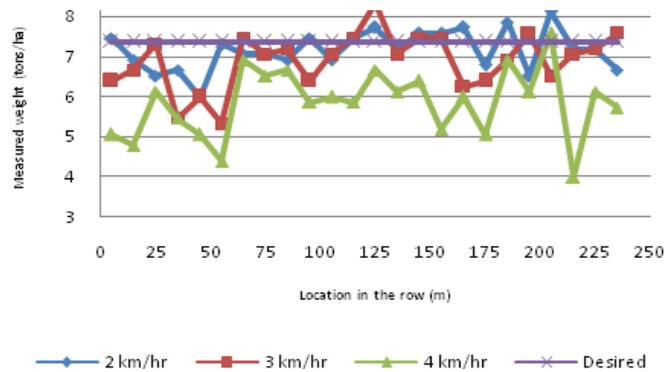
Figure 11. Comparative uniformity of planting billets at 2, 3 and 4 km hr<sup>-1</sup> forward speeds
