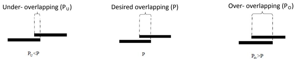
Figure 5. Billets position after being dropped on the furrows
