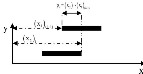
Figure 6. The method of overlap calculation
