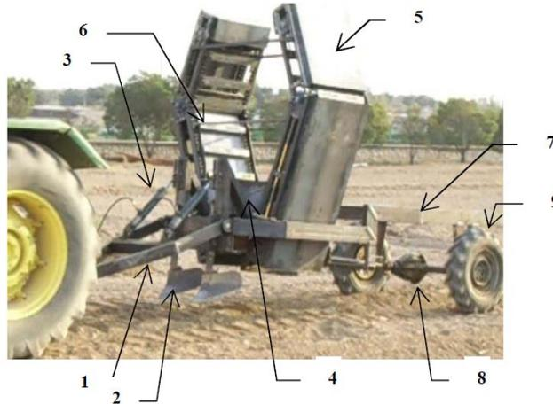
Figure 3. Different parts of evaluated billet planter: 1- Drawbar, 2- Furrower, 3- Hydraulic cylinder, 4- Billet hopper, 5- Metering unit, 6- cupboard, 7- Chassis, 8- Differential, 9- Ground wheel
