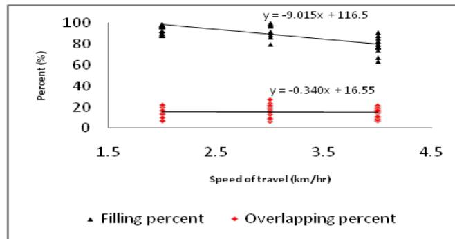
Figure 7. Graph of filling percentage changes of cupboards (triangles) and overlap pattern (diamond) affected by forward speed
