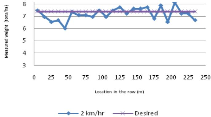
Figure 8. Uniformity of planting at 2 km hr<sup>-1</sup> forward speed compared with desired level of billet consumption
