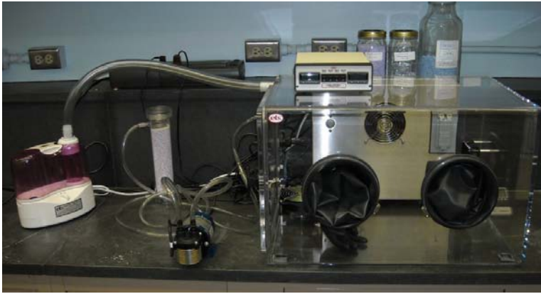
Figure 1. Controlled Environment Chamber (CEC) and associated hardware
