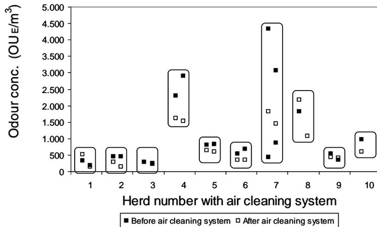
Figure 4. Odour concentrations measured before and after the air cleaners.
