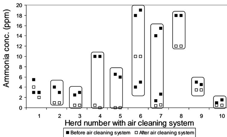
Figure 2. Ammonia concentrations measured before and after the air cleaners. Ammonia measurements were taken about 12 am and 2 pm for each herd. Herd number 3, 4 and 5 had chemical acid air cleaners from Scan Airclean A/S. The others were bio-trickling filters from SKOV A/S. In herd 6, 7 and 8 a part of the ventilation air was extracted from the manure channels, while the rest of the air was extracted through a duct in the ceiling.
