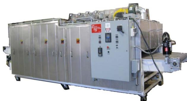
**Figure 3 Mobile infrared heating equipment for processing vegetables and fruits**
