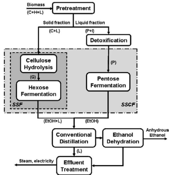
Figure 2. Generic block diagram of bioethanol production from lignocellulose biomass (Cardona Alzate and Sanchez Toro (2005))
