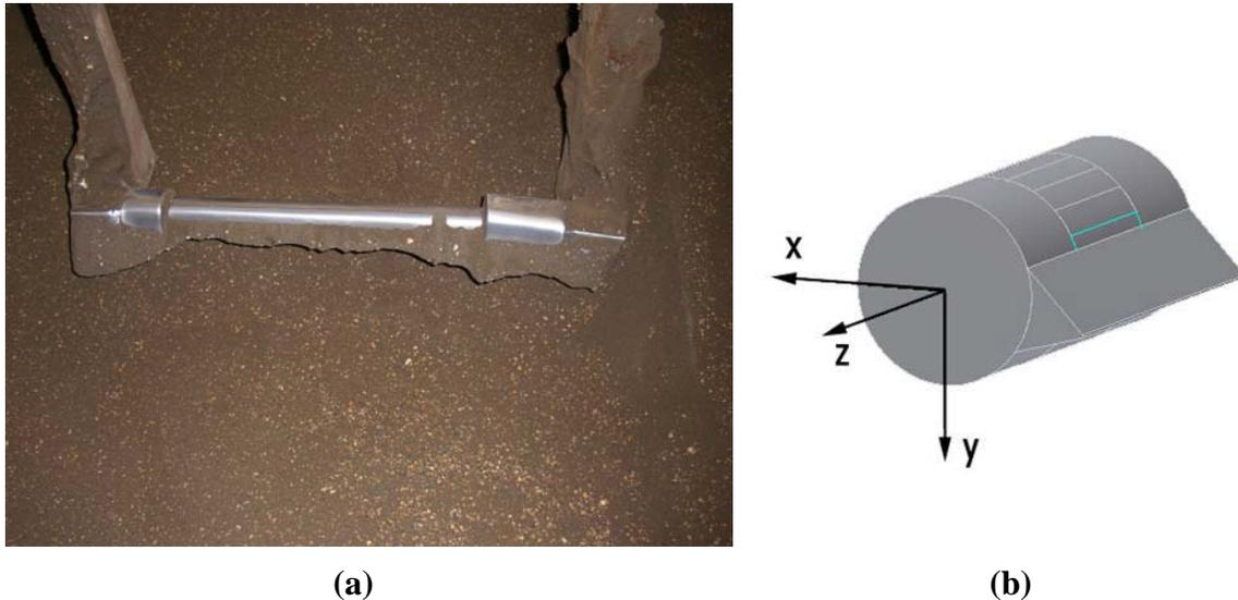
Figure 1. (a) Specimen used by Graff et al. (2009) in soil bin tests and (b) replicated geometry from simulations.
