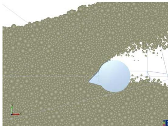
Figure 3. Screenshot of bar as it passes through the simulated soil bin.
