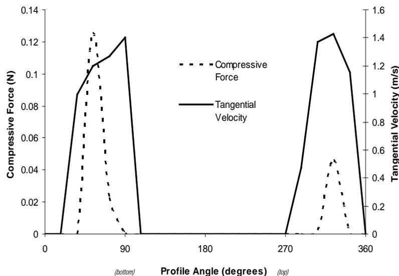
Figure 4. Distribution of simulation generated compressive force and tangential velocity on the bar profile.
