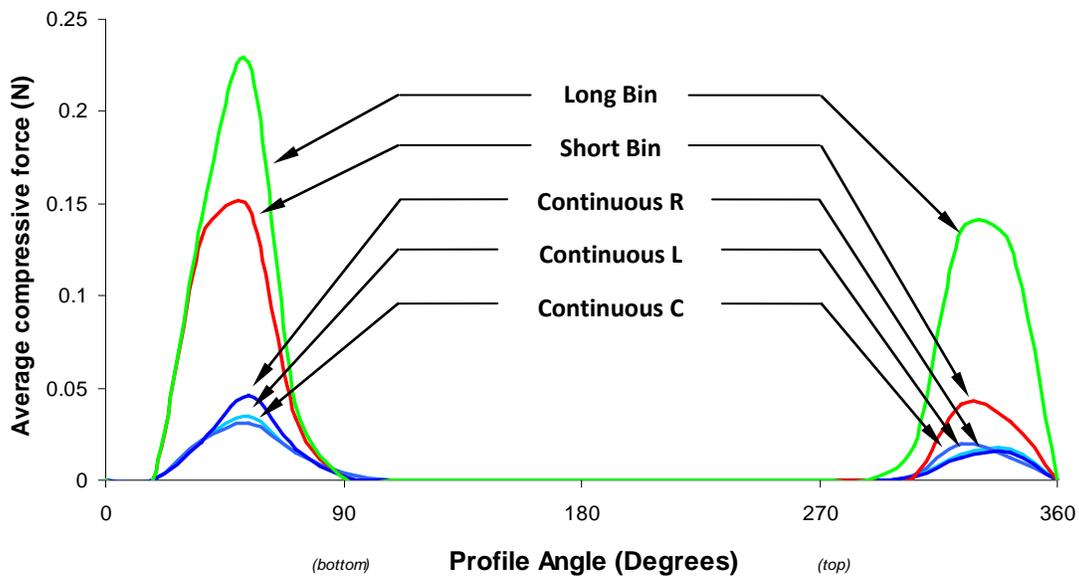
Figure 7. Distribution of simulated compressive forces for initial bar with original, longer, and continuous bins at the left (Continuous L), center (Continuous C), and right (Continuous R) locations.
