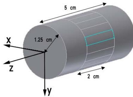
Figure 2. Diagram of tool used in simulation.
