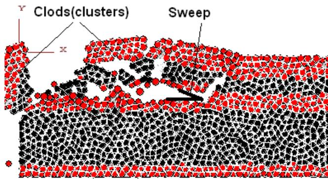
Figure 15. Soil-Tool Interaction by DEM model
