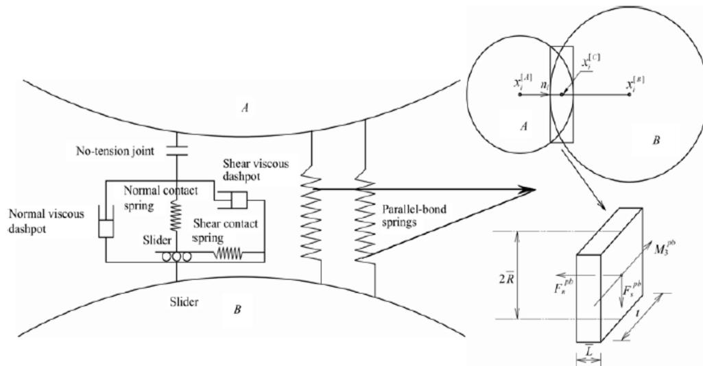
Figure 6. The nonlinear mechanical model of contact between soil particles.
