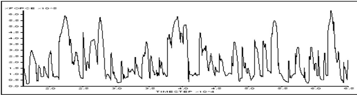
Figure 13. Draft force (N). Speed: 4,6 m/s. Result of a shear process.
