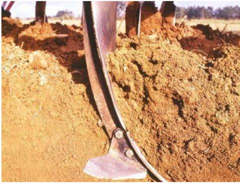
Figure 14. Soil-Tool Interaction in cohesive soil
