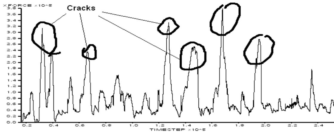
Figure 11. Draft force (N). Speed: 0,6 m/s. Result of a shear process, with the cracks marked.
