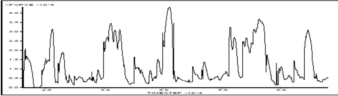
Figure 12. Draft force (N). Speed: 2,6 m/s. Result of a shear process.
