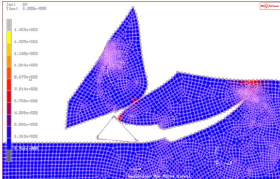
Figure 2. The VCCT method in FEM as the Soil-Tool Interaction in cohesive soil.
