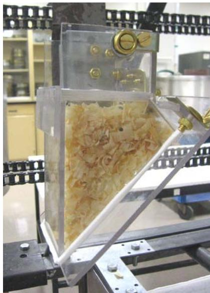
Figure 1. Specially designed acrylic container filled up with a carrier material (thin wood chips in this case), a water soaked tampon, and 50 *P. Maculiventris* 2<sup>nd</sup> instar nymphs.
