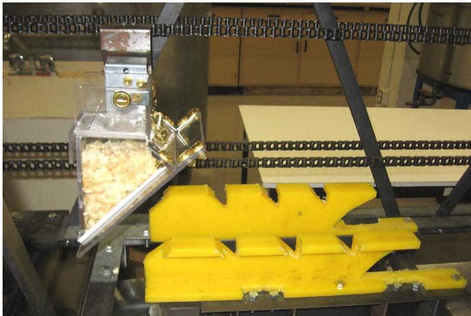
Figure 2. Specifically designed acrylic container mounted on a chain conveyor of the laboratory test bench to simulate the mechanical release of predators in potato crops. Diagonal notches were done in both sides of the release tracks to shake down the nymph predators that would remain inside the container.
