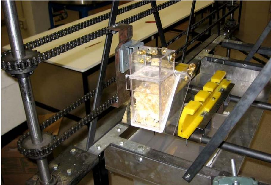
Figure 3. Overview showing the container, the yellow release system, and the tray underneath the release zone in which fall down the carrier material and the predators.
