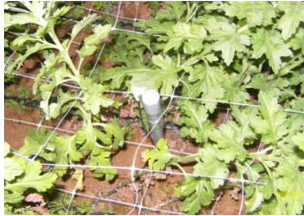
Figure 4. Tensiometer installed in greenhouse (laying depth 20 cm)
