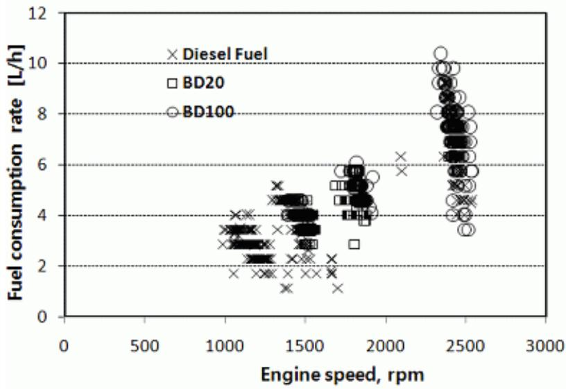
Figure 3. Engine RPM and fuel consumption rates by the different fuels.
