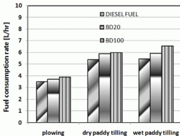
Figure 4. Fuel consumption rate by the different paddy operations.
