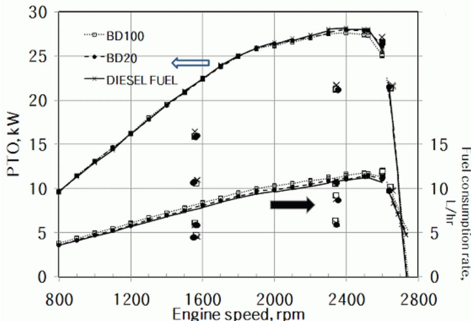
Figure 2. Engine speed, fuel consumption rate and PTO output.
