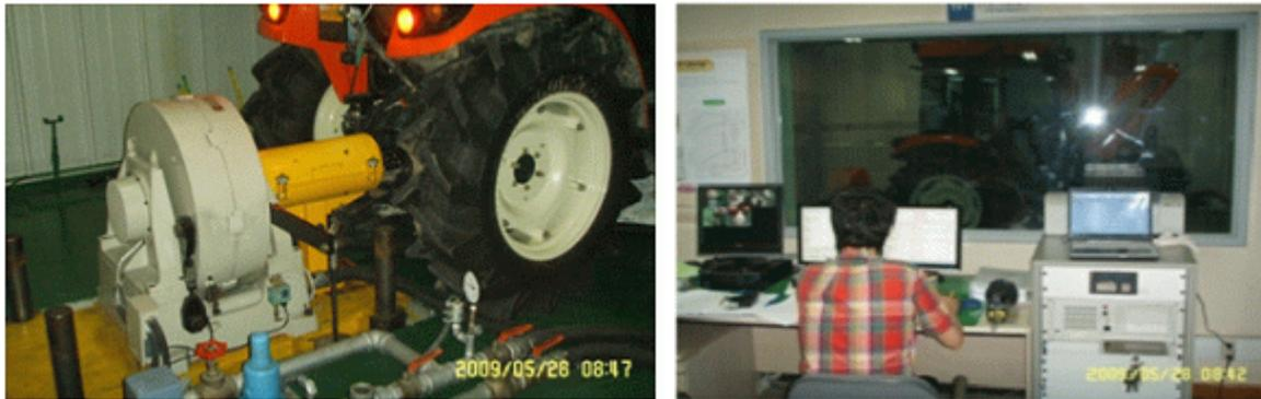
Figure 1. PTO performance test.
