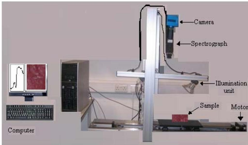
Figure 1: A laboratory NIR hyperspectral imaging system.
