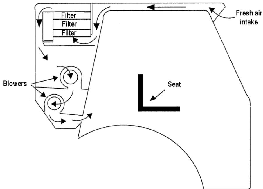
Figure 1. Schematic description of a typical cab filtration system (Adapted from Heitbrink et al., 1998)
