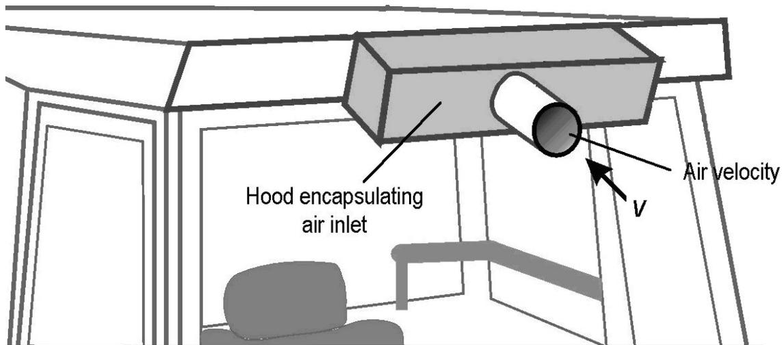
Figure 2. Example of blocked filter unit with hood encapsulating nominal air inlet and array to measure air flow velocity (Adapted from Hinz, 2008)
