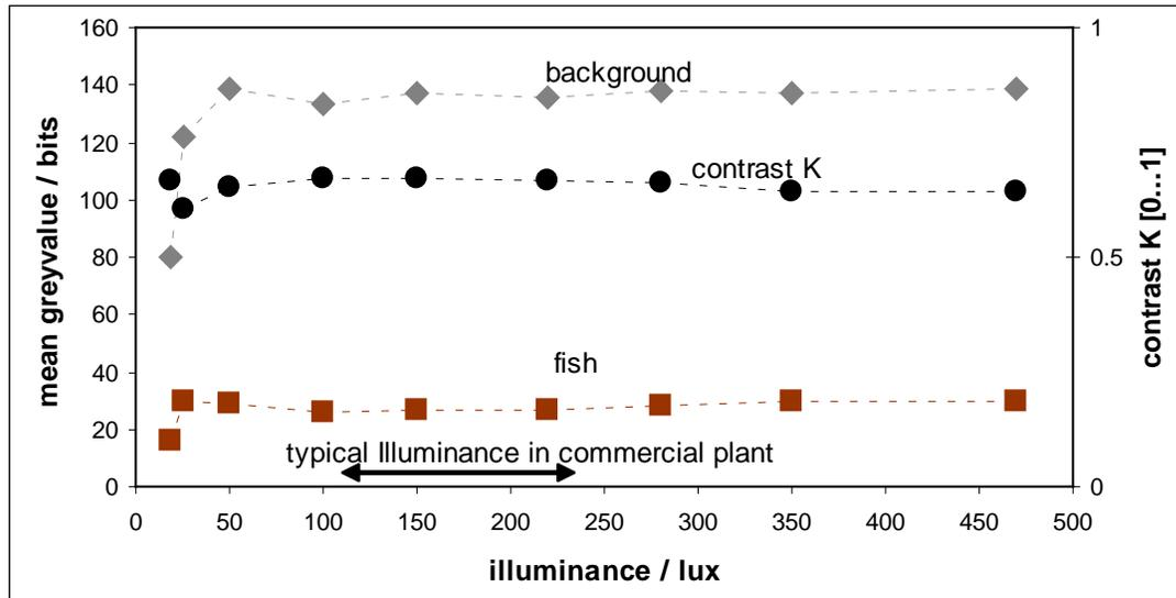
Figure 4. Contrast at different illumination.
