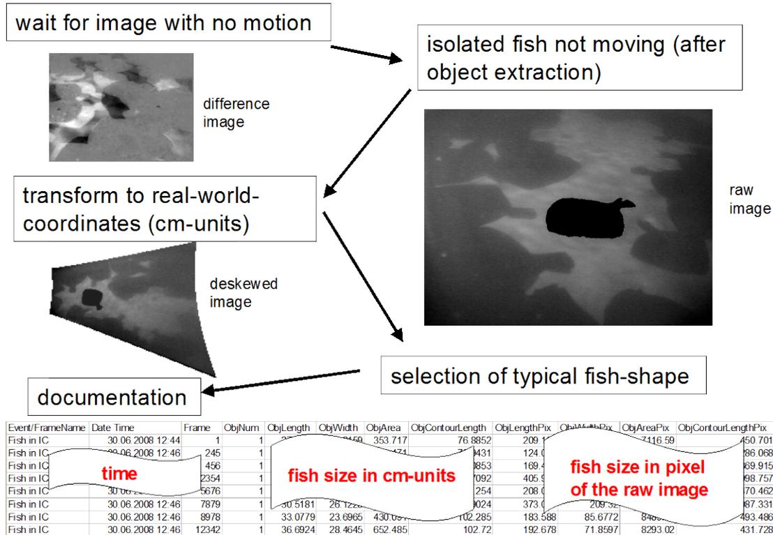
Figure 2. The algorithm of image analysis in principle.
