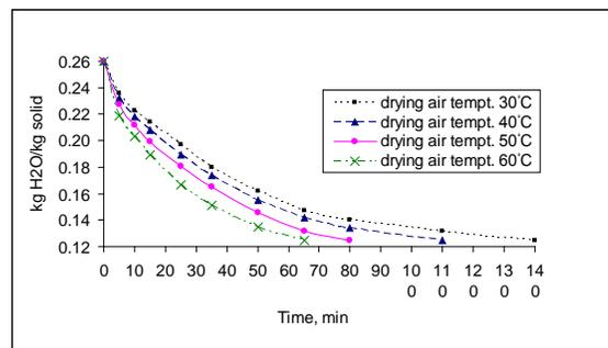
Figure 4 Effect of drying air temperature on drying time of shelled corn without microwave radiation energy
