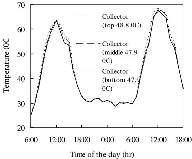
Figure 3. Temperature profile in vertical direction of collector section of the tunnel.
