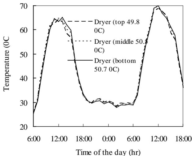
Figure 4. Temperature profile in vertical direction of dryer section of the tunnel.
