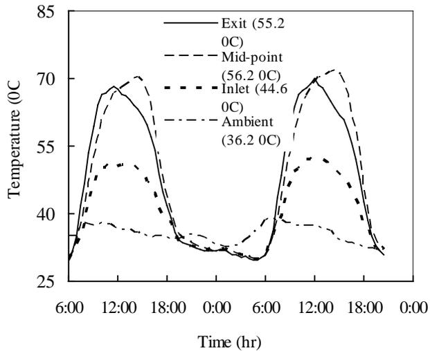
Figure 5. Variations of ambient, dryer and collector temperatures with time of the day (July 27-28, 2009,) in drying freshly harvested dates.
