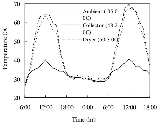
Figure 2 Variations of ambient, dryer and collector air temperatures with time of the day (August 8-9, 2008) under no load condition.
