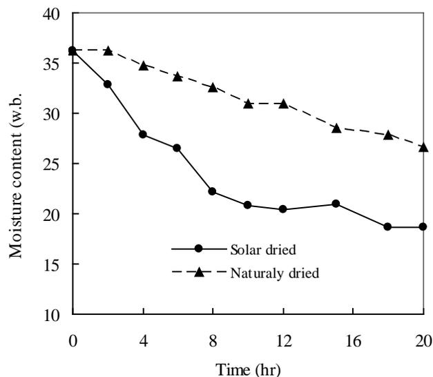
Figure 7. Variations of moisture content with drying time with solar tunnel dryer and natural open air sun drying
