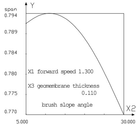
Fig. 11. Influence of the brush slope angle on the effect of paving
