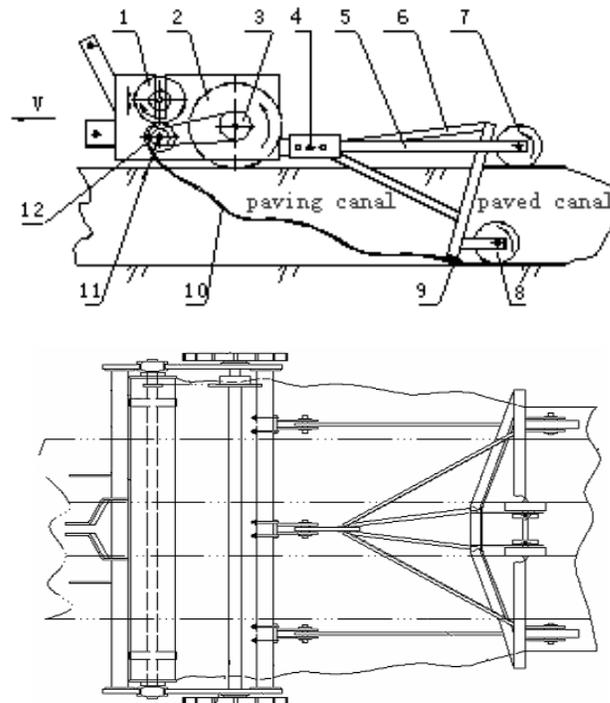
1. geomembrane roller 2. driving wheel 3. chain wheel 4. connecting mechanism 5. presser rod 6. brush rack
