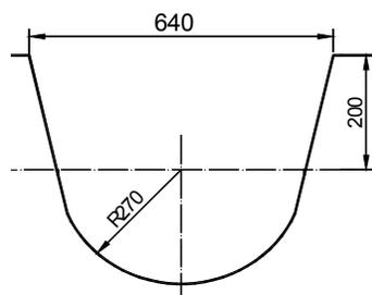
Fig. 5. The size of the canal base
