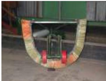
Fig. 4 The structure of U brush
