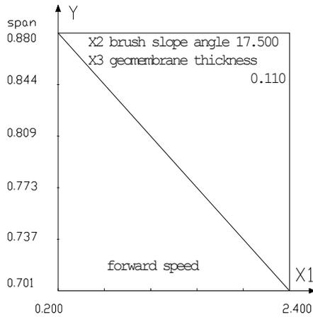
Fig. 10. Influence of forward speed on paving effect
