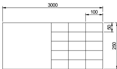
Fig. 2. Calibrated geomembrane net
