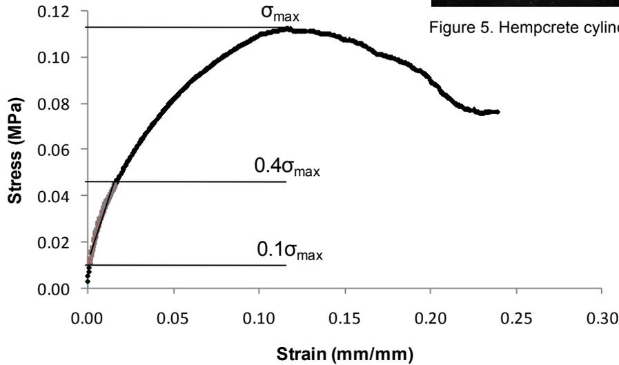
Figure 4. Stress-strain data for specimen 15 from binder mix LCF101
