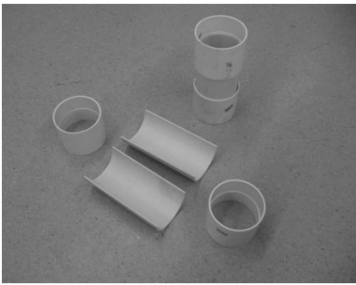
Figure 2: Breakaway mold
