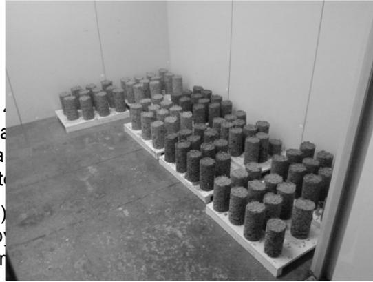
Figure 3: Curing of test cylinders
