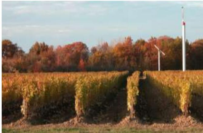
Figure 1. Wind machines are used worldwide to protect crops against cold injury.
