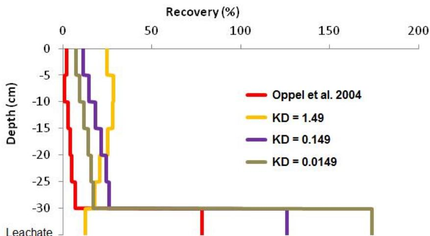
Figure 5. Observed (Oppel et al., 2004) and predicted iopromide transport with varying  $K_D$ .
