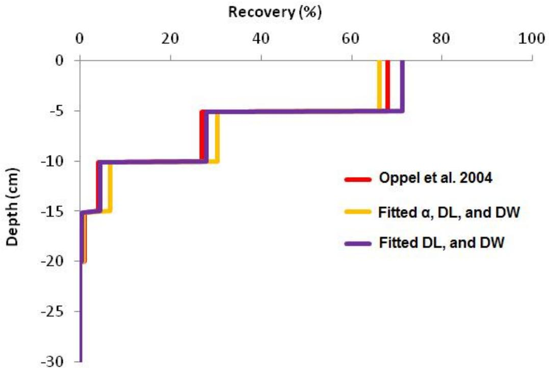
Figure 4. Final fitted data for diazepam using inverse solution to fit  $\alpha$ ,  $D_L$  and  $D_W$ , and using a fixed  $\alpha$  and fitted estimates for  $D_W$  and  $D_L$ , in comparison to data from Oppel et al. (2004).
