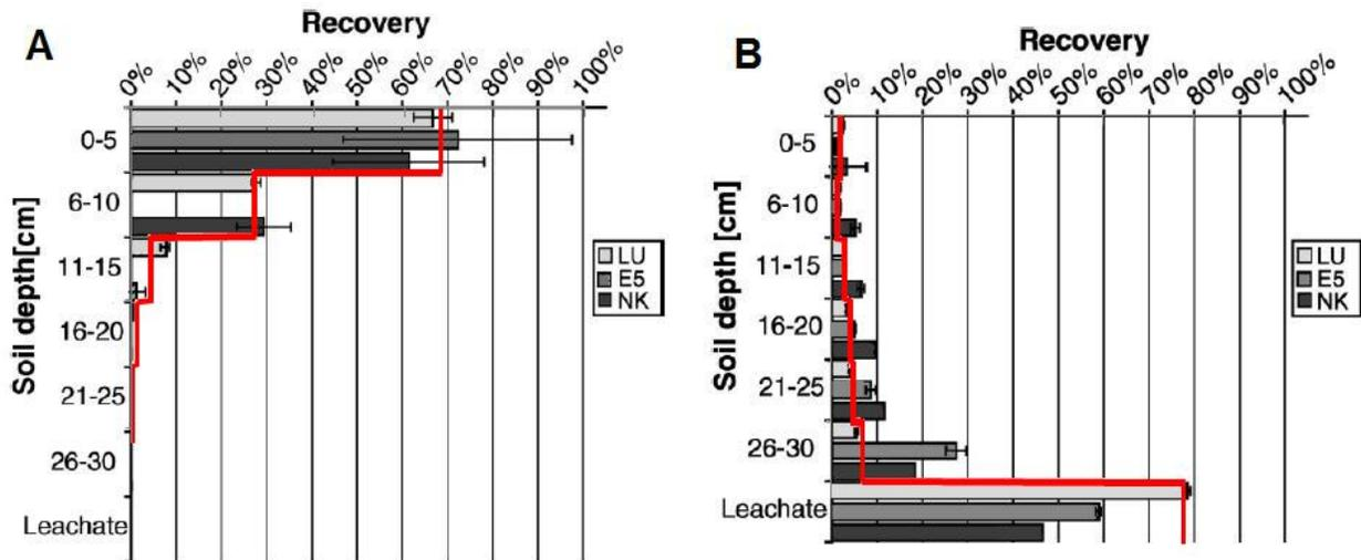
Figure 1. Data reproduced from Oppel et al. (2004) describing the concentration of diazepam (A) and iopromide (B) in the soil profile and leachate from a soil column study. The line represents the extracted values used in modelling.
