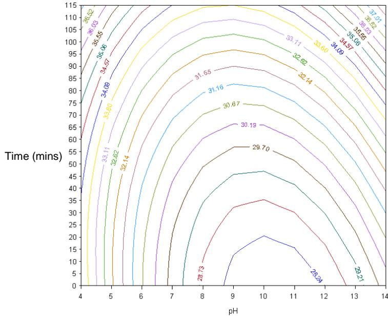
Figure 2: Contour plot of dry matter separation values at percentage of biochar 6%
