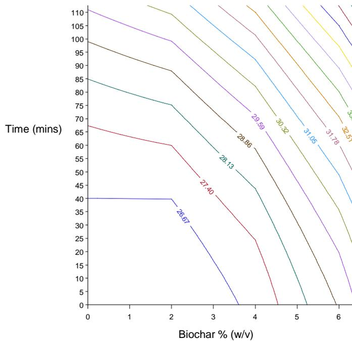
Figure 3: Contour plot of dry matter separation values at pH 13
