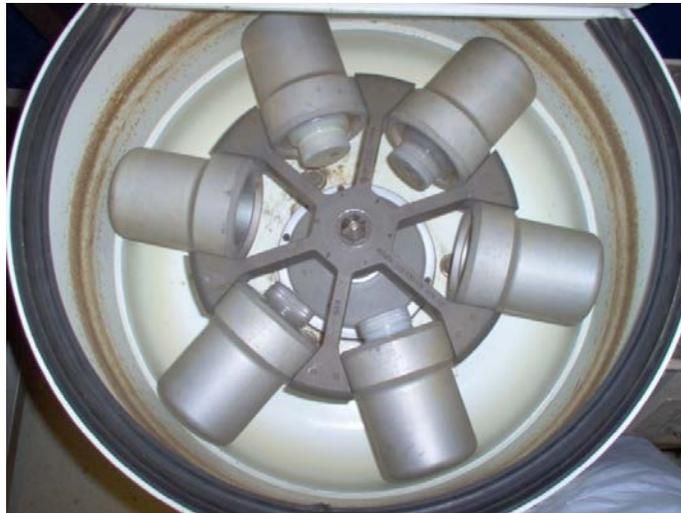
Figure 1: Laboratory centrifuge utilized for centrifugation of swine manure
