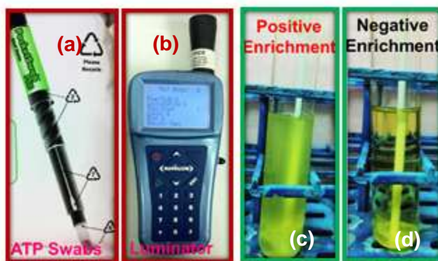
Figure 7: Sampling indicators used: ATP Bioluminescent Relative Light Unit (RLU) readings and bacteria presence enrichment data. ATP swab (a); ATP laminator (b); positive (turbid) bacteria enrichment (c); negative bacteria enrichment (d).
