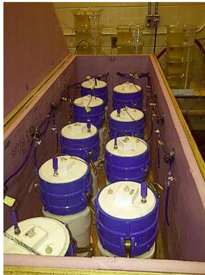
Figure 1: Incubator set-up with 9 vessels
