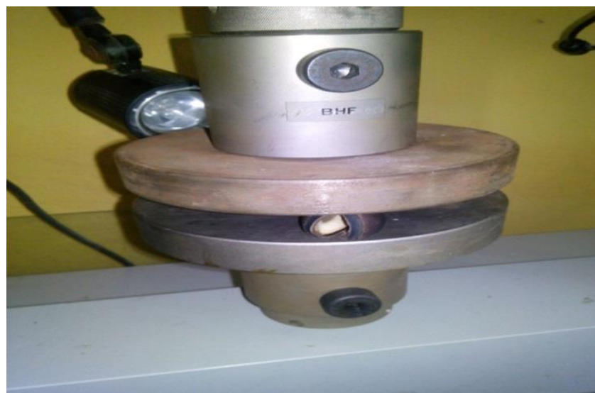
Figure 2: Cracking of mucuna bean seed by compression using a UTM
