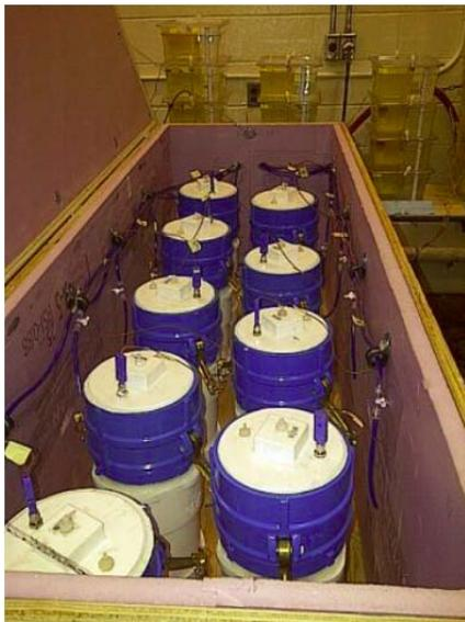
Figure 1. Incubator set-up with nine vessels. Two incubators are used for a total of 18 vessels.
