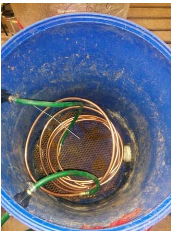
Fig 4. Copper tube heat exchanger
