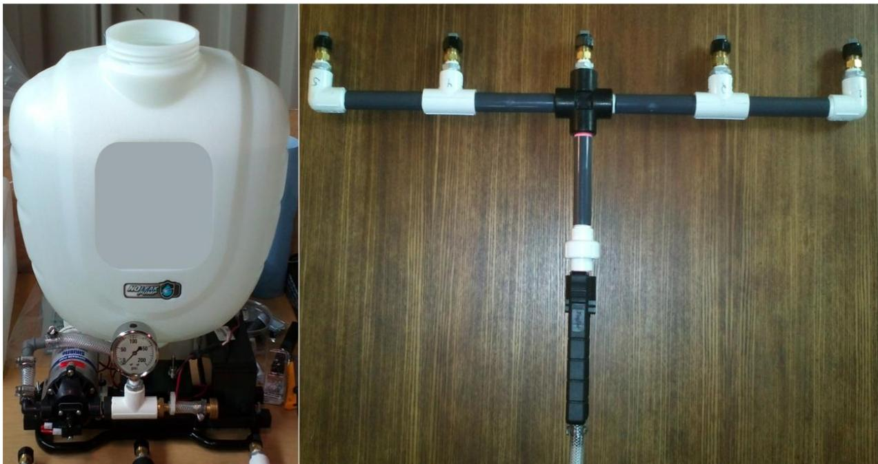
**Figure 1.** Left side: modified backpack sprayer with diaphragm pump and battery. Right side: five nozzles spraying boom.
