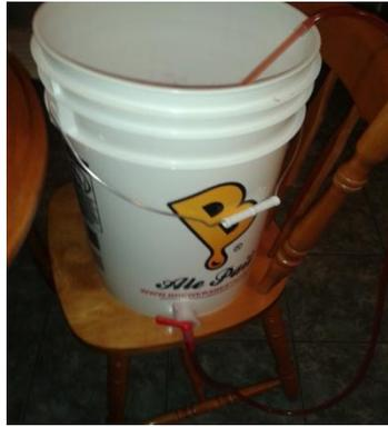
*Figure 8: The bottling bucket with attached spigot and bottle filler (left).*
