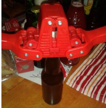
Figure 10: A 355mL bottle of beer being capped using a dual hinge capper.
