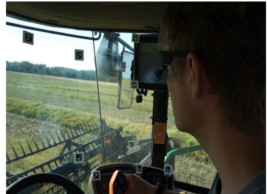
Figure 5. Operator monitoring the right side of the header; the GPS unit is obstructing the view.
