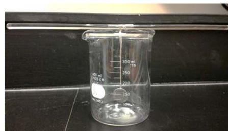
Figure 2. Vertical wicking apparatus
